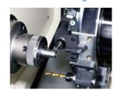
CNC Precision Turning Center This is a process-intensive, complex machine that enables both turning and milling processes. Combining a lathe and a machining center, this machine can handle a wide range of machining demands without changing the settings.
