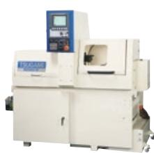
This machine tools are fitted to minimize any effects resulting from high temperatures, and its cast iron base, with high rigidity, can suppress the vibration that occurs during high-speed processing. Hence, it enables stable and accurate processing for a long time.
